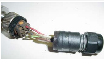
Corroded EXV Cable Connector
